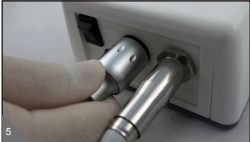
Finishing the connection of motor cord and control box
